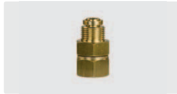
3/8" AG : 1/4" IG. Messing. Max. 220 bar / 90 °C
