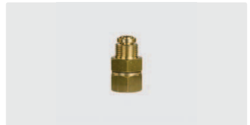
3/8" AG : 1/4" IG. Messing. Max. 220 bar / 90 °C
